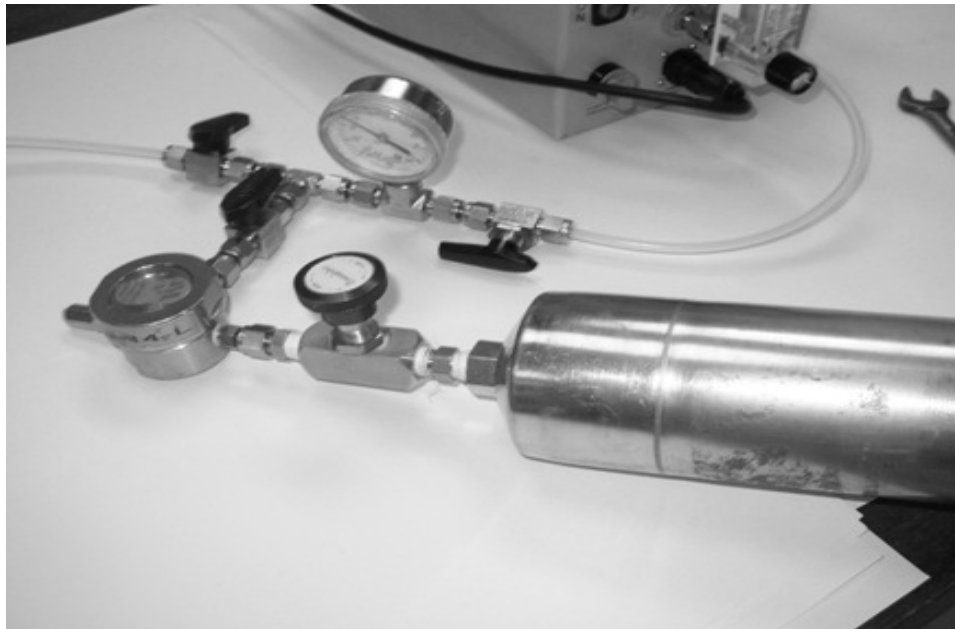
FIGURE 1 Sampling Manifold
