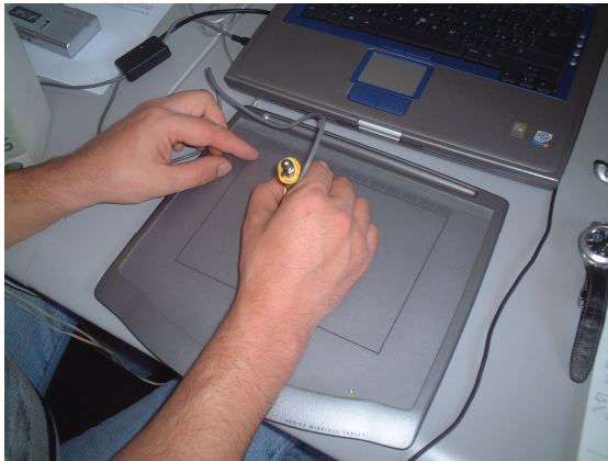
Fig. 3. Experimentation of the AudioTact® device: a visually impaired user explores the virtual image using the left hand for spatial references and the right hand for scanning for aural and vibrational cues
